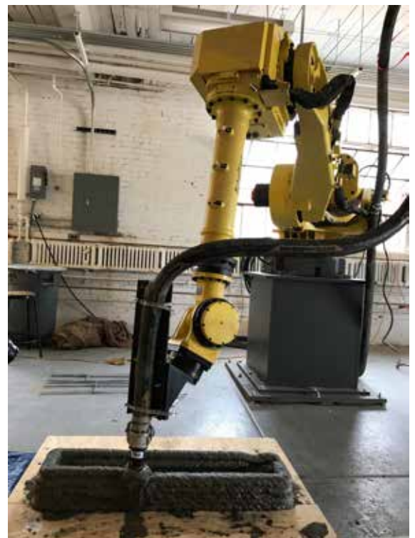
Fig 3. Robotic Arm Configured for Concrete Printing
