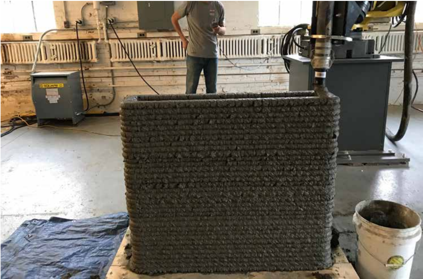
Fig 4. Steel-reinforced 3'x3'x8" Concrete Printed Wall
