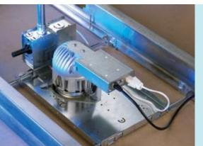
Renaissance Lighting's solid-state fixtures are as easy to install as incandescent or fluorescent fixtures. Our user-friendly design includes a simple two-wire system and a mounting frame with cross-bar hangers for easy installation in framed or suspended ceilings.
