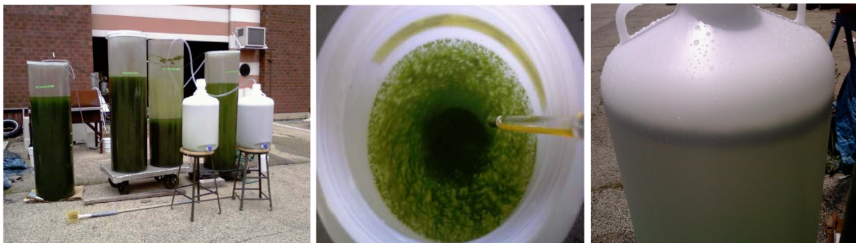
Figure 5. Algal cells can be harvested from the modular bioreactor system (left) using chemical flocculating agents that cause the cells to aggregate (middle) and settle rapidly out of solution (right).
