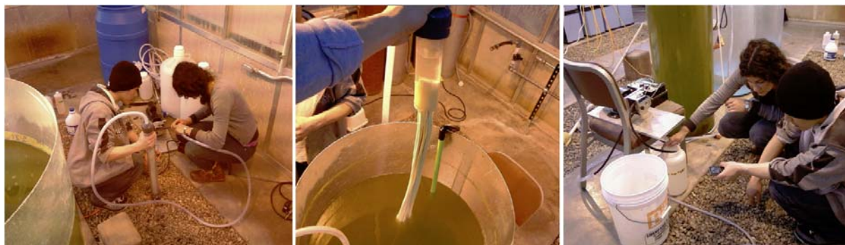
Figure 6. The membrane harvest unit (left) consists of a series of micro-porous tubes bound together (middle) that allow water to pass through while retaining the algal cells. The water can then be recycled for future growth cycles (right).
