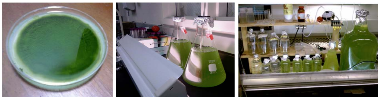
Figure 1. Algal strains are received on culture discs and scaled over a 10-day growth period into 2-L and 20-L laboratory flasks.
