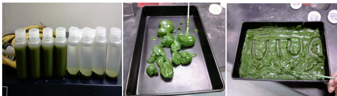
Figure 7. The harvested algal slurry (left) is further concentrated using batch centrifugation to produce cell pellets (middle). The pellets are then spread thin and oven-dried to <5% moisture prior to lipid extraction (right).
