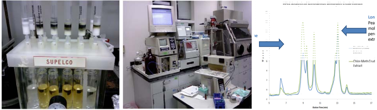
Figure 9. The composite lipid extract is separated into neutral, glyco-, and phospho-lipid fractions using solid phase extraction cartridges (left). The chemical compounds in each fraction are further identified using high performance liquid chromatography (middle and right).
