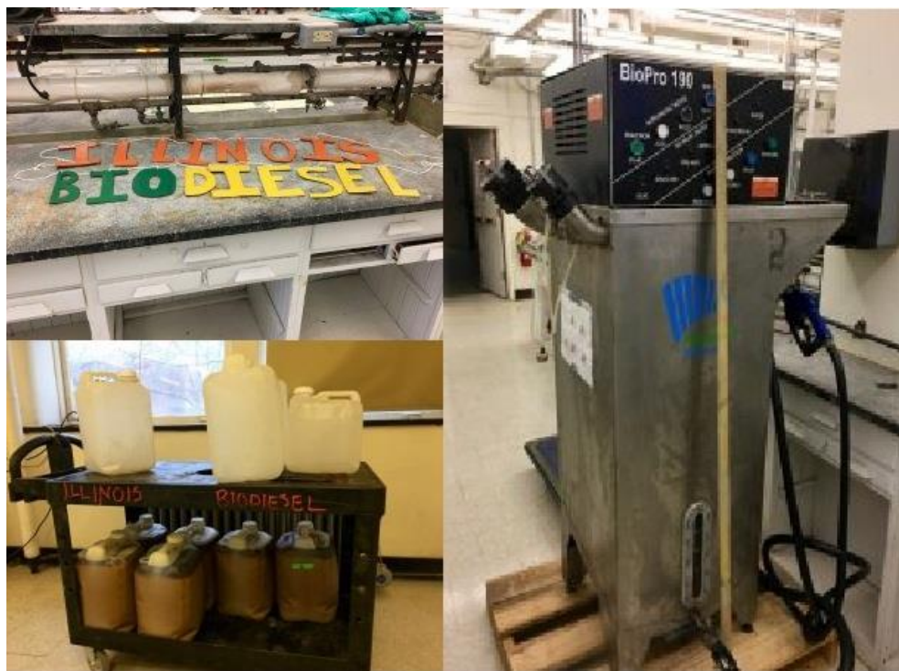
Figure A3. Oil containers from the dining hall, and the reactor that converts the waste into a final product of usable fuel. (source: http://ssc.sustainability.illinois.edu/?p=1760 )
