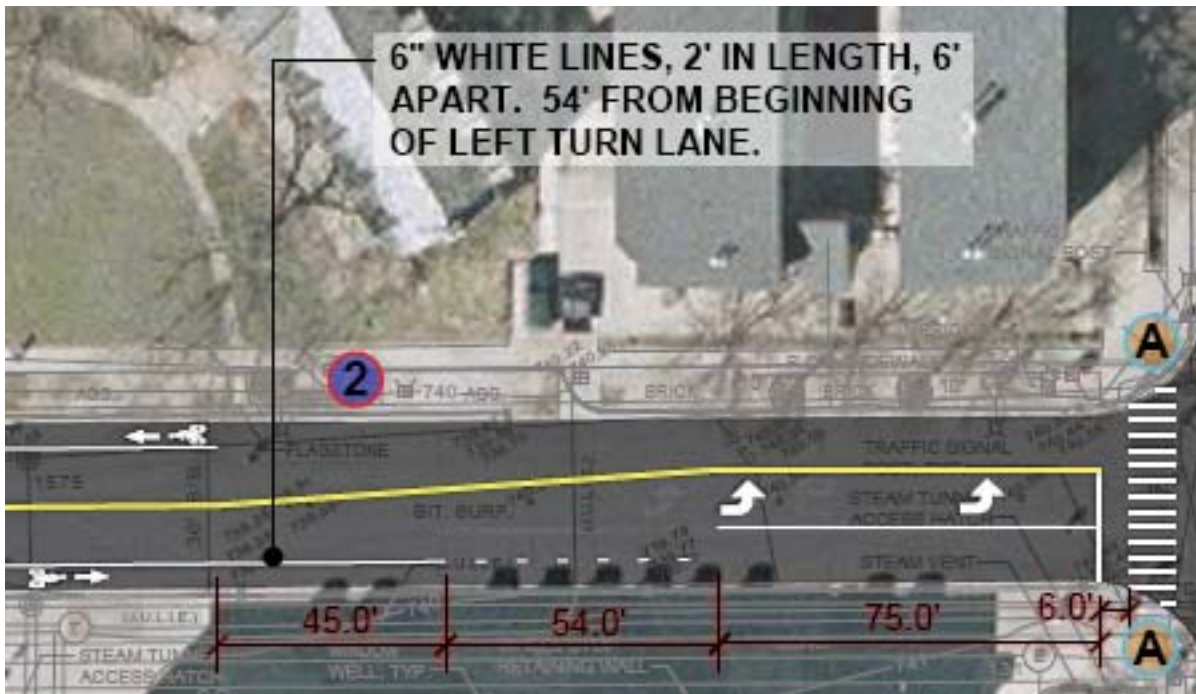
Figure 4. Bike Lane striping layout at intersection with spacing dimensions Figure by Tiffany Williams
